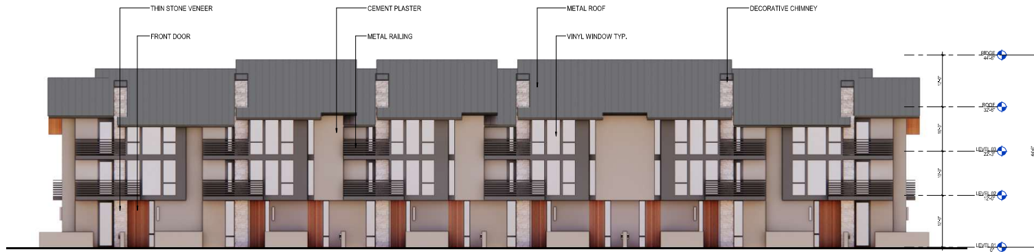
12-PLEX FRONT ELEVATION 3 SCALE: 1/8" = 1'-0"
